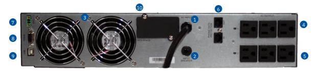
1 10 ft. Power Cord 2 Input Circuit Breaker 3 Cooling Fan 4 Load Bank 1 5 Load Bank 2 6 Phone/Network Surge 7 Remote EPO Port 8 RS-232 Communications 9 USB Communications 10 Accessory Slot
