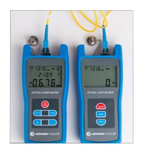
Designed to measure both the absolute optical power and relative power loss in fiber optic cables. These power meters feature the following:
