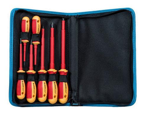
Jonard's 7 Piece Insulated Screwdriver Kit contains 3 Phillips and 4 Slotted screwdrivers, which are made of chrome vanadium steel with a black oxide finish and are heat treated for maximum strength and durability. These screwdrivers meet or exceed IEC 60900, ASTM F1505-01, and VDE standards for high voltage protection and are tested to 10,000 VAC and rated to 1,000 VAC live use. This kit includes:
